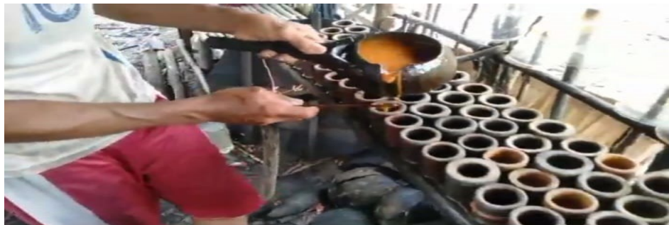
Gambar 3 Proses pencetakan Gula Aren
