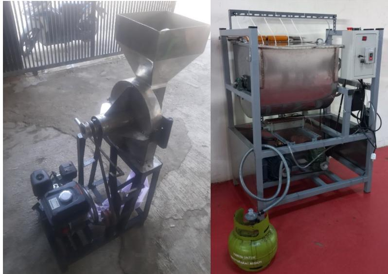
**Gambar 6. Hasil Fabrikasi Mesin (a) *Sugar Grinder* (b) *Powder Mixer***
