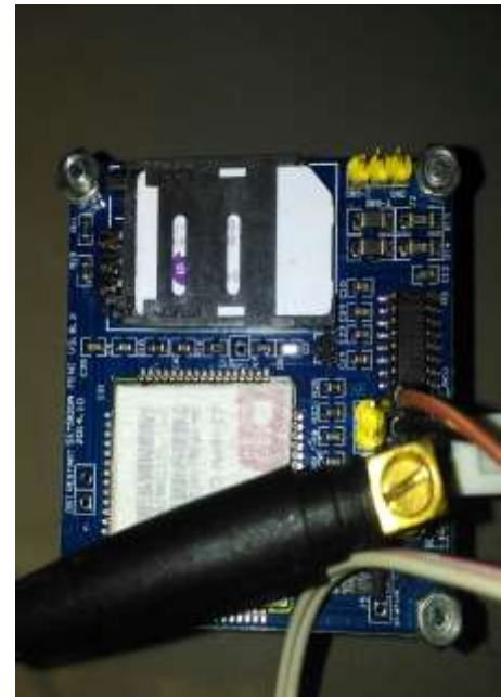
Gambar 4.2 Sim Card Terpasang di Modul GSM
