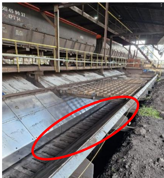
Figure 2. Example Lining Stainless stell at hopper apron feeder
