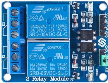
Gambar 4 Module Relay 2 Channel
