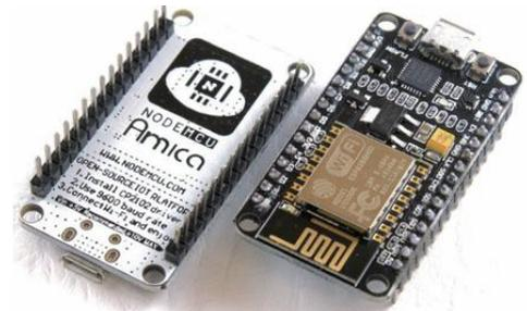
Gambar 3 NodeMCU ESP8266
