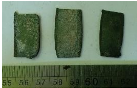
Gambar 1. Sampel Paduan Titanium Hasil Pengerolan
