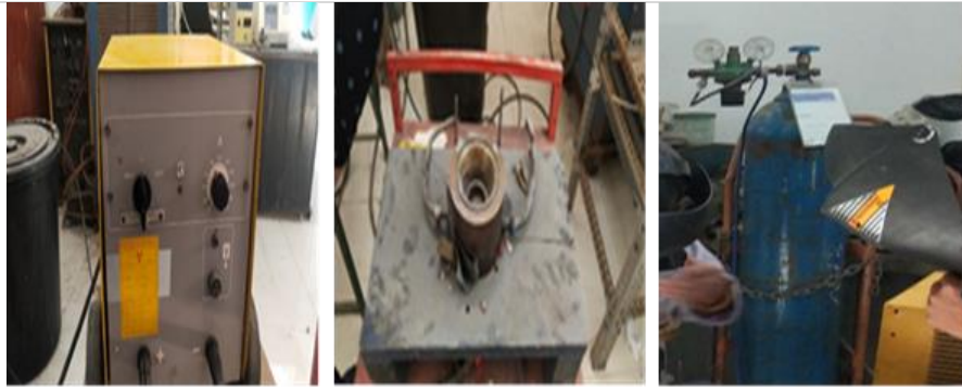
Gambar 3. Alat Peleburan Single Arc Melting Furnance Sumber : (Dokumen pribadi)
