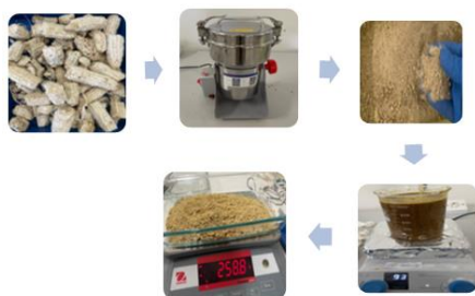
Figure 3. Flow Chart of Procedure Used for Cellulose Extraction
