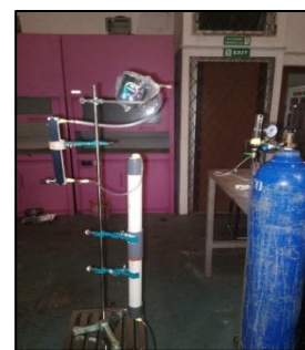
Figure 1. Adsorption Tools Combined (Adsorber Column, Gas Flow meter, and Gas Tank)
