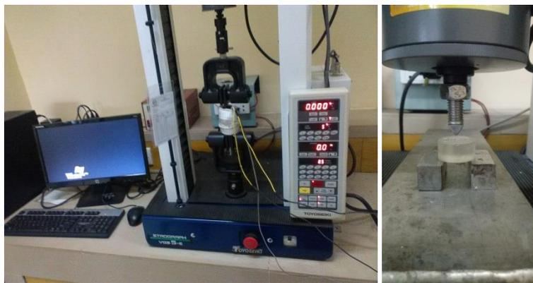
**Gambar 2.** (a) Alat Universal *Testing Machines* Kapasitas 5 KN
