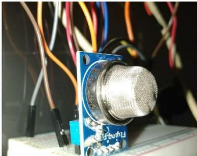
Gambar 14 Tampilan Sensor Gas MQ-6
