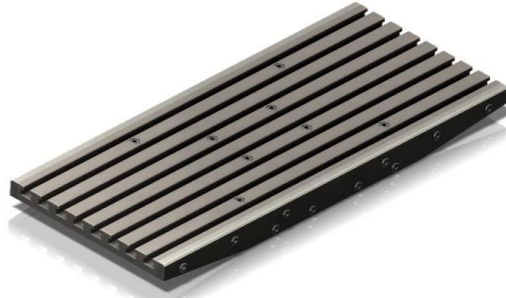
Gambar 2. Desain Bed Machine Milling CNC 3 Axis
