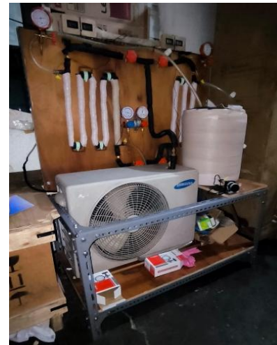
Gambar 4. Alat Air Conditioner Water Heater
