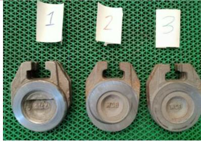
Gambar 1. Spesimen Uji *disc overlay gate valve*
