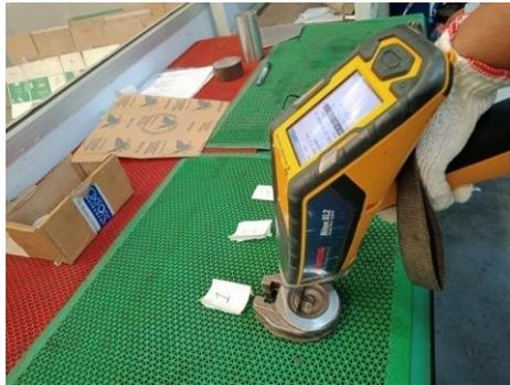
Gambar 3. Pengujian PMI (Positive Material Identification)
