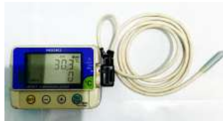
Gambar 5. Digital thermometer HIOKI LR5011.
