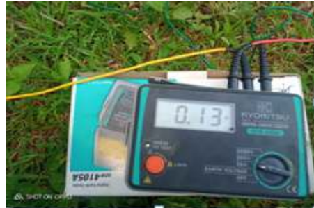
Gambar 6. Pengukuran Pentanahan Lab EMC
