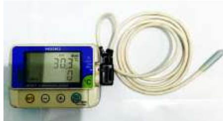
Gambar 5. Digital thermometer HIOKI LR5011.
