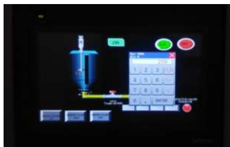
Gambar 14. Tampilan HMI tangki mixing dan konveyor counter.
