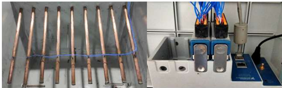
Gambar 7. Integrasi termokopel evaporator Ni 9213 cDAQ9185.
