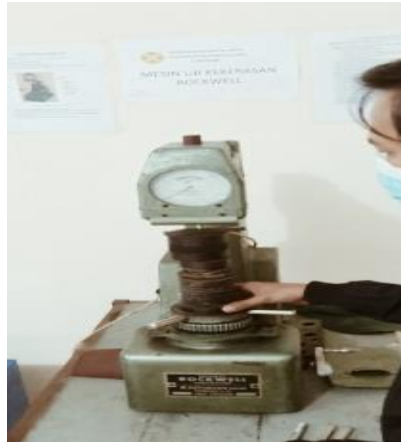
Gambar 3.4 Proses uji kekerasan Hardness rockwell
