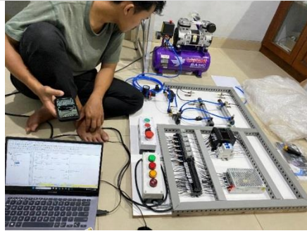
Gambar 19. Proses Validasi Program PLC
