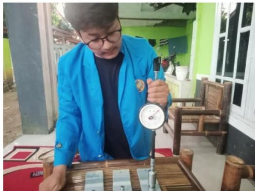
Gambar 11. Proses Uji Tarik/Bonding Material Cat
