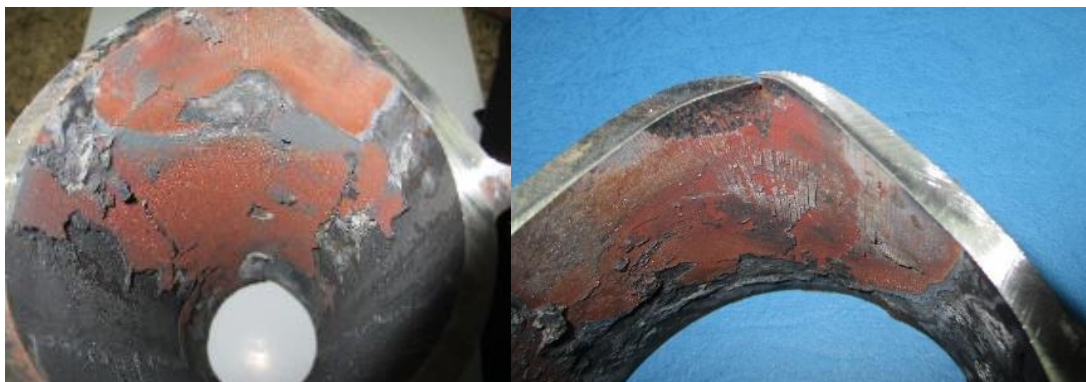
Figure 4. Thick deposit can be observed on inner surface of tube
