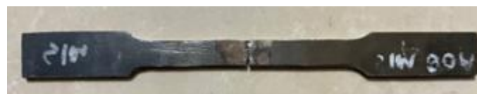
Figure 6. Fractured photographs of tensile specimen of GTAW with welding consumable of ST 37
