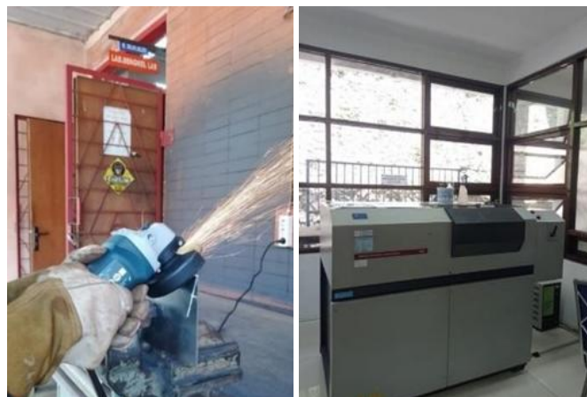
Figure 1. Butt-weld joint preparation with 30° of bevel angle (left), The ARL optical emission spectrometer machine (right)
