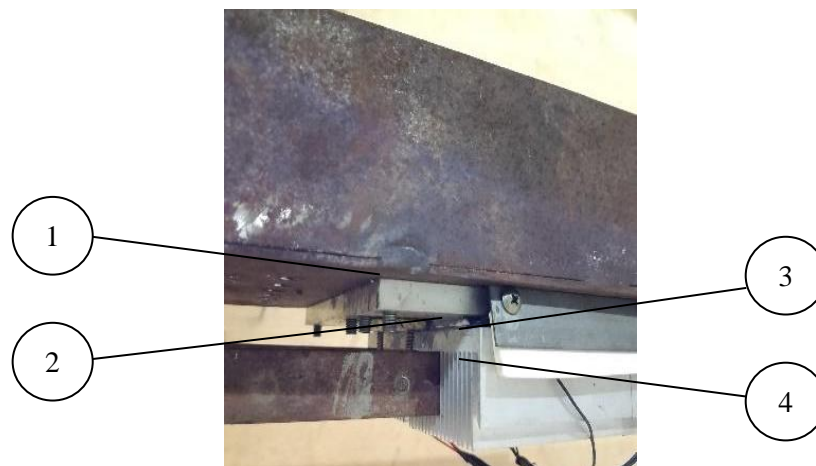
Figure 6. Temperature sensor mounting point on the satay grill
