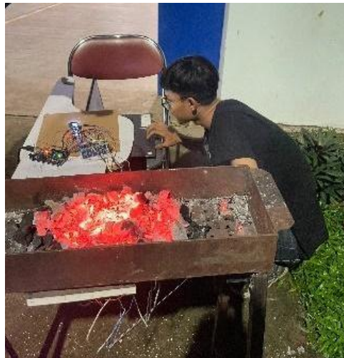
Figure 5. Testing the satay grill with a data acquisition set
