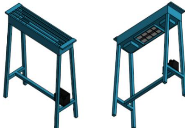
Figure 2. Satay Grill Design: a). Top view, and b). Bottom view
