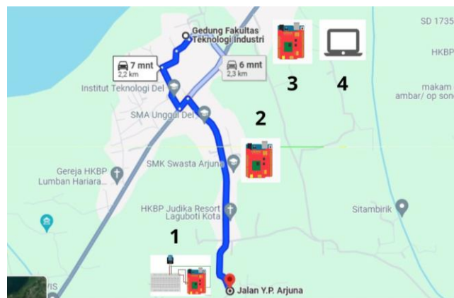
Figure 6. Multihop scenario in LoRa network 1=Transmitter Node, 2= Repeater, 3= Gateway, 4=Serial Monitor
