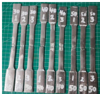
Figure 6. Tensile test result at varying welding current 30, 40 and 50 A
