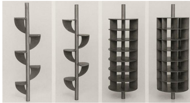
Figure 3. Variations in quarter-circular blade numbers with 2, 4, 8, and 16 blades [6], [16]–[18]
