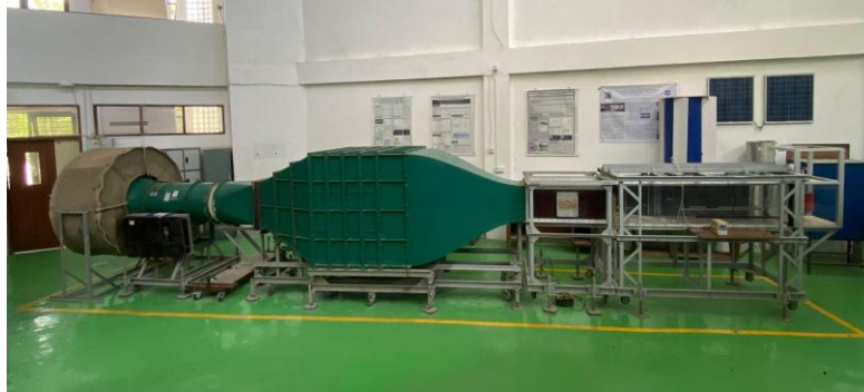
Figure 6. Experimental setup of the Flettner-VAWT rotor in the wind tunnel. Source: Laboratory documentation
