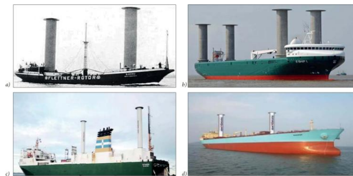
Figure 1. Example of Flettner rotor installation on a maritime vessel [2]
