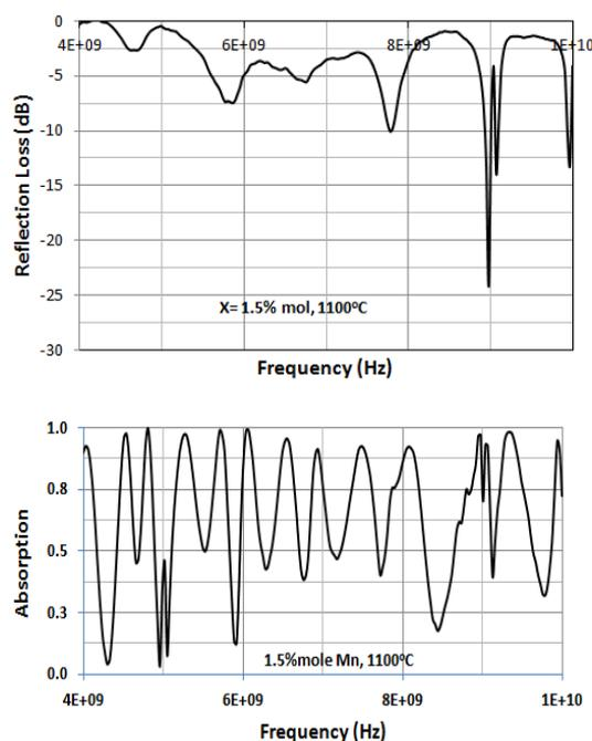
Figure 7. a). Correlation of reflection loss (RL) as a function of frequency and b). Absorption as a function of frequency on  $\text{BaFe}_{10.5}\text{Mn}_{1.5}\text{O}_{19}$  magnet.
