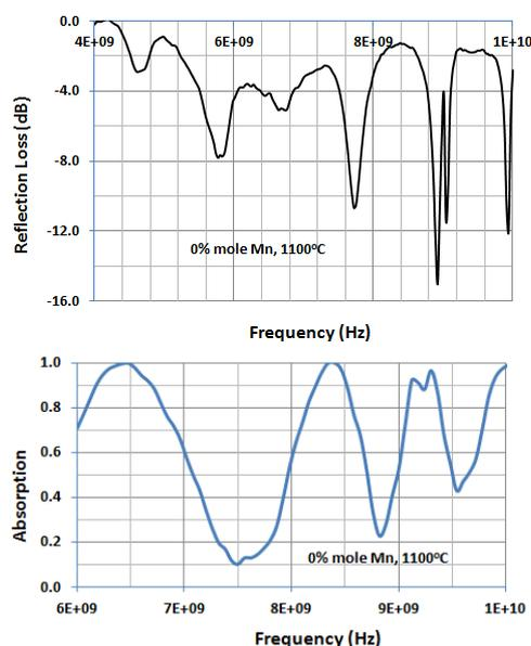
Figure 6. a). Correlation of reflection loss (RL) as a function of frequency and b). Absorption as a function of frequency on  $BaFe_{12}O_{19}$  magnet.
