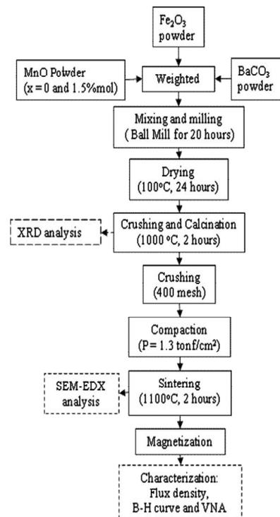
Figure 1. Flowchart of sample preparation and characterization of  $\text{BaFe}_{(12-x)}\text{Mn}_x\text{O}_{19}$  magnet.
