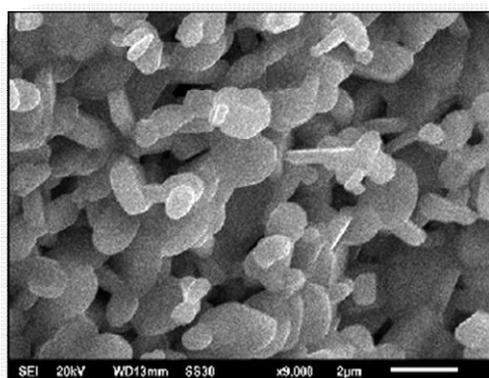
Figure 3. Scanning Electron Micrographs (SEM) analysis of  $BaFe_{12}O_{19}$  magnet after sintered at temperature of  $1100^{\circ}C$  (2 hours).
