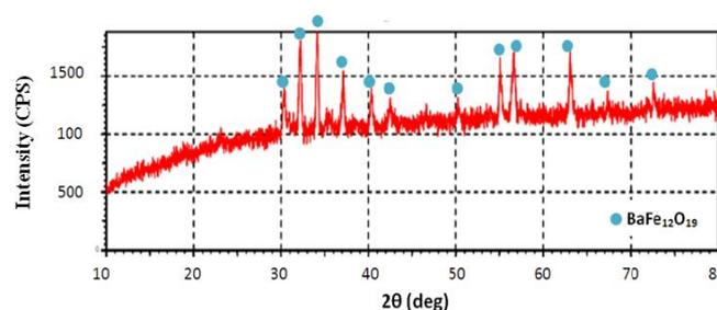
Figure 2. XRD curve of  $\text{BaFe}_{12}\text{O}_{19}$  material after calcination process at the temperature of  $1000^\circ\text{C}$  for 2 hours.
