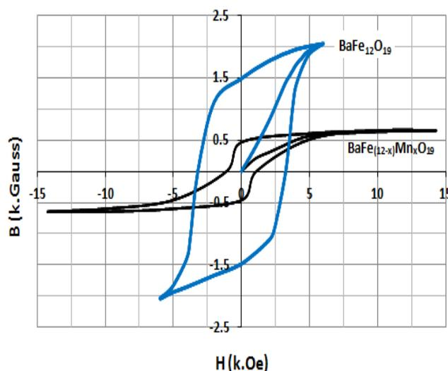
Figure 5. Magnetic hysteresis loops of  $\text{BaFe}_{12}\text{O}_{19}$  and  $\text{BaFe}_{10.5}\text{Mn}_{1.5}\text{O}_{19}$  after sintered at the temperature of 1100°C (2 hours).
