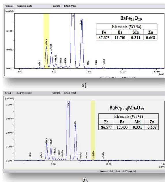
Figure 4. Micro X-Ray Fluorescence ( $\mu$ XRF) analysis, a).  $BaFe_{12}O_{19}$  hard magnet and b).  $BaFe_{10.5}Mn_{1.5}O_{19}$  magnet
