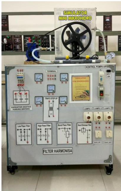
Fig. 2. The final product of micro hydro generation simulator
