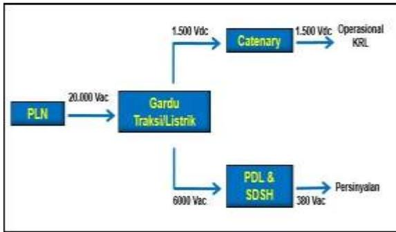
**Figure 2.** Conversion of overhead electric power [2].
