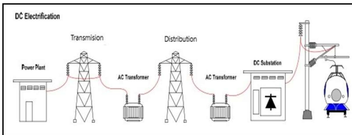
Figure 1. Distribution of KRL electrical power [2].
