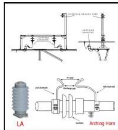
**Figure 4.** OHGW on catenary grid [3].
