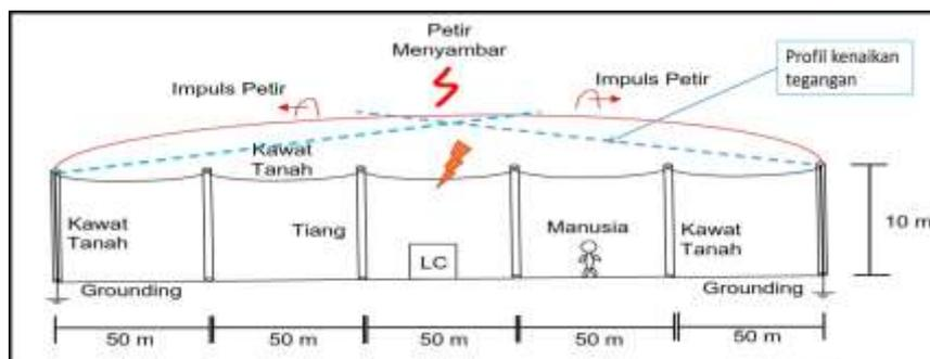
**Figure 13.** Illustration of an existing pole at the time of a lightning strike.
