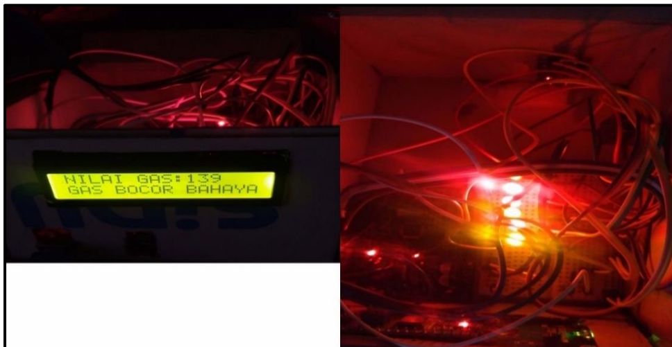
Gambar 3.2 Tampilan Lampu 1-6 menyala Gas Bocor, Buzzer & kipas On
