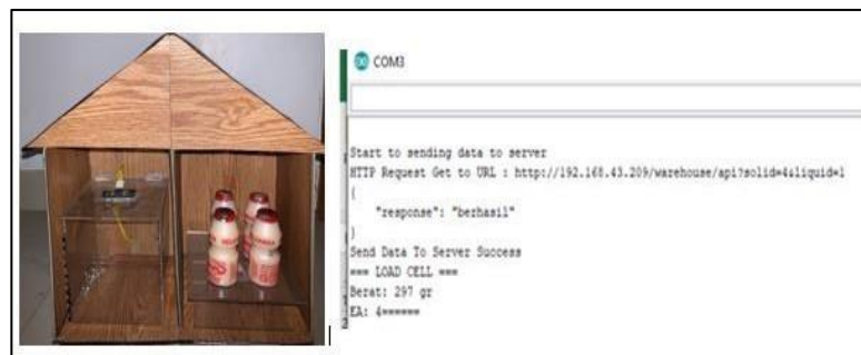
Gambar 13 Proses Pengujian Sensor Load Cell
