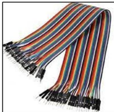
Gambar 8. Kabel Jumper
