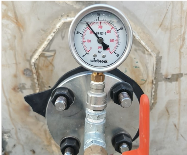
Gambar 1.5 Hydrotest Heating Coil sampai Tekanan 15 Bar
