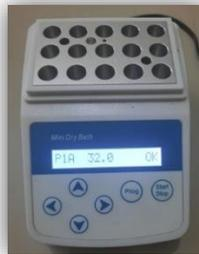
Gambar 2. Kalibrator thermometer (Mini Dry Bath)
