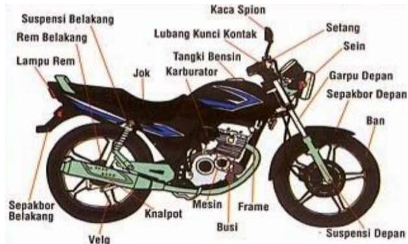
Gambar 1. 1 Unit sepeda motor
