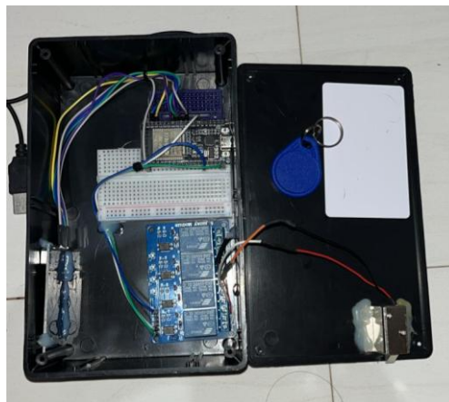
Gambar 3. Prototipe Sistem Smart Keyless 2FA Berbasis ESP32, RFID RC522, Telegram Bot, Relay, dan Solenoid Lock
