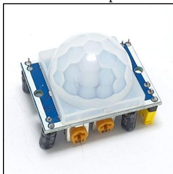
Gambar 4. Sensor PIR HC-SR501
