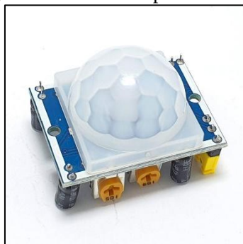
Gambar 4. Sensor PIR HC-SR501
