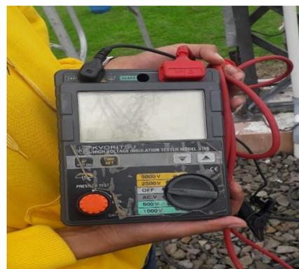
Gambar 6. Alat ukur *Insulation Tester*
