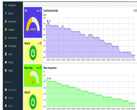
Gambar 12. Tampilan dashboard thinger.io monitoring TDS relay ON
