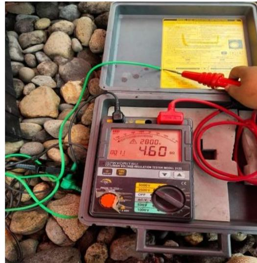
Gambar 5. Insulation tester merk kyoritsu
