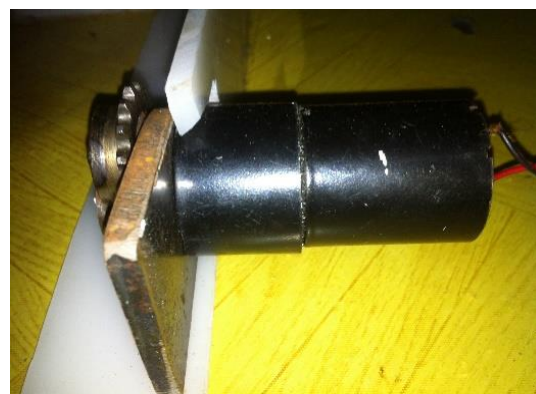
Gambar 8. Motor DC 12-24 V
