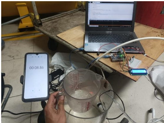
Gambar 7. Proses kalibrasi alat monitoring debit air
