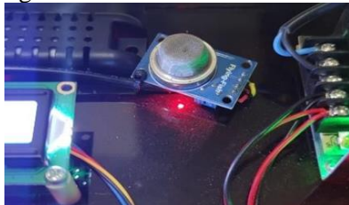
Gambar 3 tampilan sensor asap MQ-2
